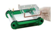
**HU13-SS** - 13cm long Scie-Plas Super-Seals offer total versatility in casting, allowing the gel length to be tailored to each user's personal requirements
