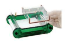
**HU10-SS** - 10cm long Scie-Plas Super-Seals offer total versatility in casting, allowing the gel length to be tailored to each user's personal requirements
